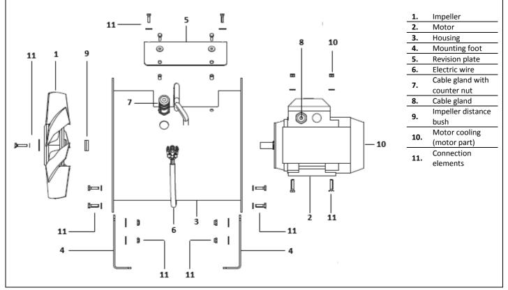
Fan housing, revision plate, mounting foots (3, 4, 5) alre made from painted steal. Impeller baldes and hub are made from aluminum. Impeller distnace bush is made from stainless stel, conection elements are made from galvanized steal. Fan casing is sealed with EPDM tape.
